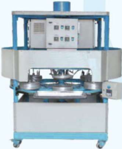
Semi Automatic Khakhra Roasting Machine
